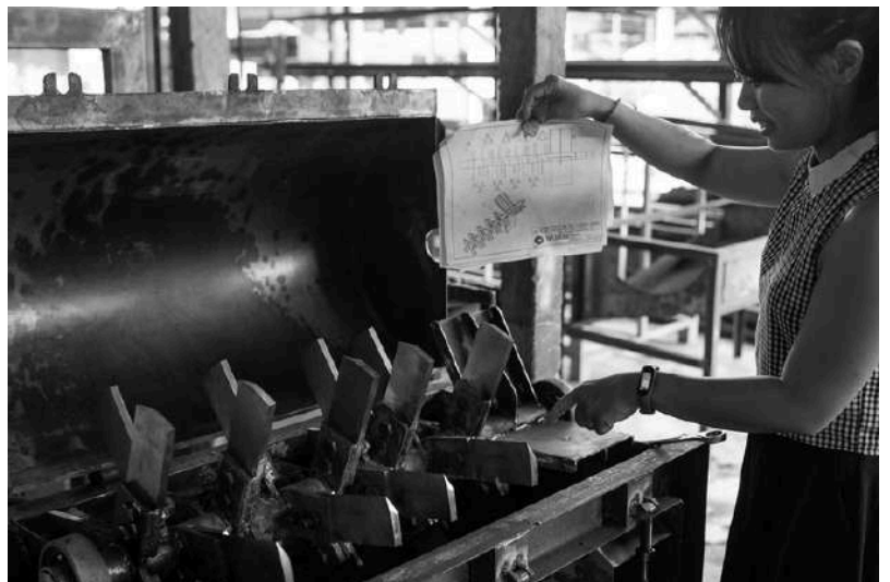
Replacable blades inside the Organic Crusher, shredding organic waste into smaller pieces and preparing them for composting or further treatment. / Photo credit: WeDoo
